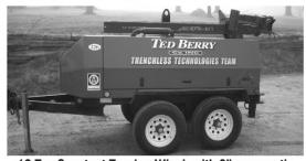
12 Ton Constant Tension Winch with 8" pneumatic hammer. For bursting municipal sewer lines made of VCP, CP, AC ect. Our HG12 Uses Patented Manhole exit.
