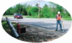
**MGD-2002 - Tracer Gas Leak Detector**
